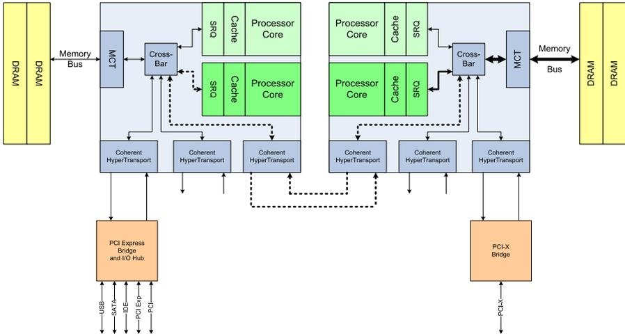
**Fig. 17** Contention of main memory requests on *Opteron*. All data are stored on a single memory node (*right bank*). As a result, one core needs to perform remote memory accesses (*dashed line*), which eventually lead to contention on the common memory controller and memory bus (*bold line*)
