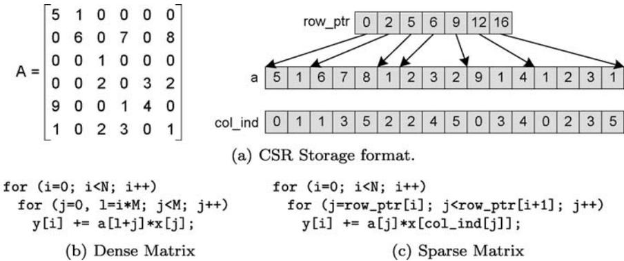
**Fig. 1** Example of the CSR storage format, dense and sparse matrix-vector multiplication kernels
